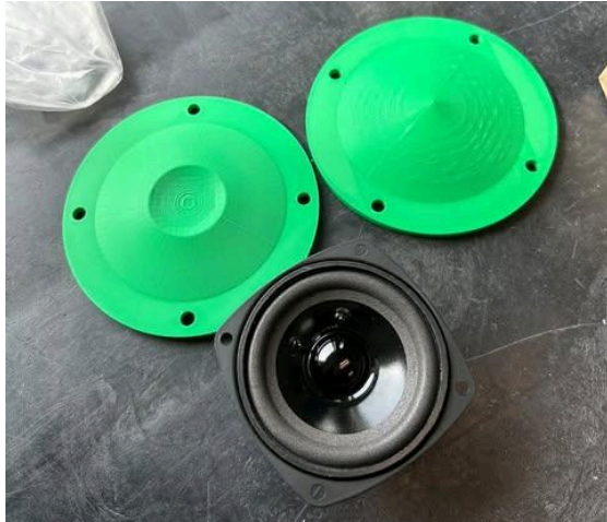
Fig 2. 3D-printed diffusers (conical and indented version) alongside the speaker driver.
